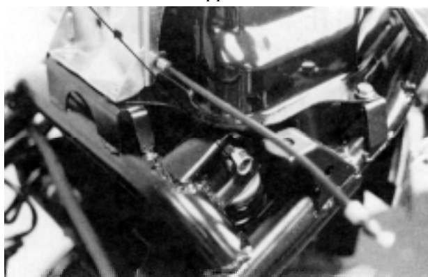
Rear Shock Absorber Upper Mount Bolt
